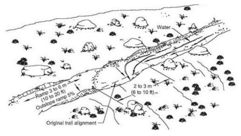
the design of a new trail, though they can also be installed in existing trails, but they require some design work and planning. They are best placed where natural dips occur or where trails curve around large trees or rocks. Smaller, simpler versions of rolling grade dips are called knicks (described earlier on page 16) and are commonly added to existing trails.
