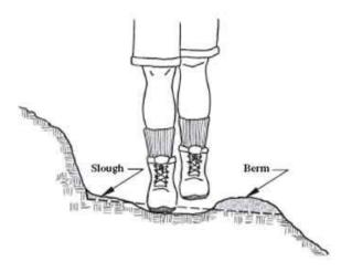
A trough has formed in the center of the trail between the "slough" and "berm."
