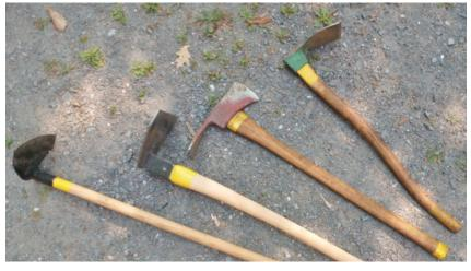
edge of a hoe can also be used to chop small roots in your way.
